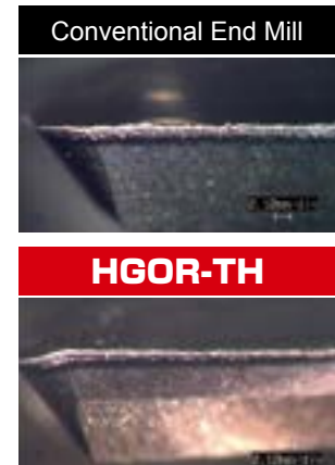
Photograph of wear after cutting 98.43 feet
