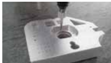
Needle contact-point mounting example
