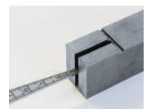
Measurement of gap width
