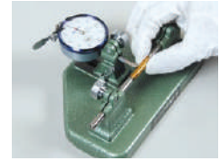
Measurement example for swing of round bar.
