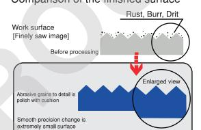
\*I can be adjusted by the roughness of the grinding wheel
