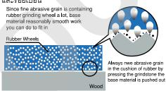
Quick polish surface reach abrasive grains to the recess while leaving the microscopic details western processing surface to cushion becomes smooth. Moreover, the accuracy varies very little because the convex portion renains. I can be adjusted by the granularity of the grinding wheel.
