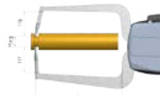
Hb Measuring contact movable Hf Measuring contact fixed L Measuring depth
