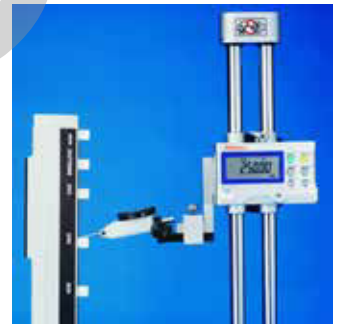
Checking accuracy of height gage
