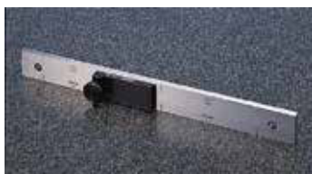
Coupling holes in long gauge blocks
