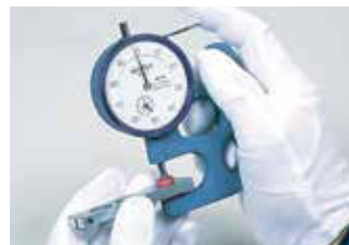
Measuring metal work piece. The photo shows 5.98mm.
