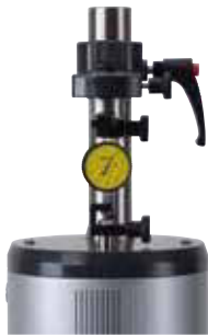
Using dial test indicator attachment set (02ASK000)
