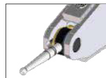
Old design: Stylus bearing screw held in frame.
