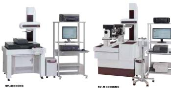
(Surface Roughness Tester with movable Y-axis column unit.) (The photo represents a special specification model.)
