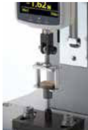
Sticking plaster adhesion test with MED-IS-20N
