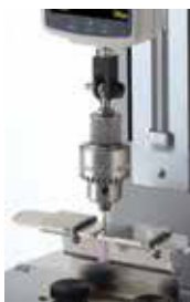
Needle pull out strength test with MED-NPT-200N
