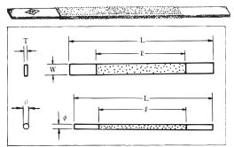
Although a special file has many kinds, I manufacture the size W, T, T, I, L, t as ordered. In addition, since I manufacture not only Common type but the triangular whole surface and quadrangular whole surface etc., please contact me.
